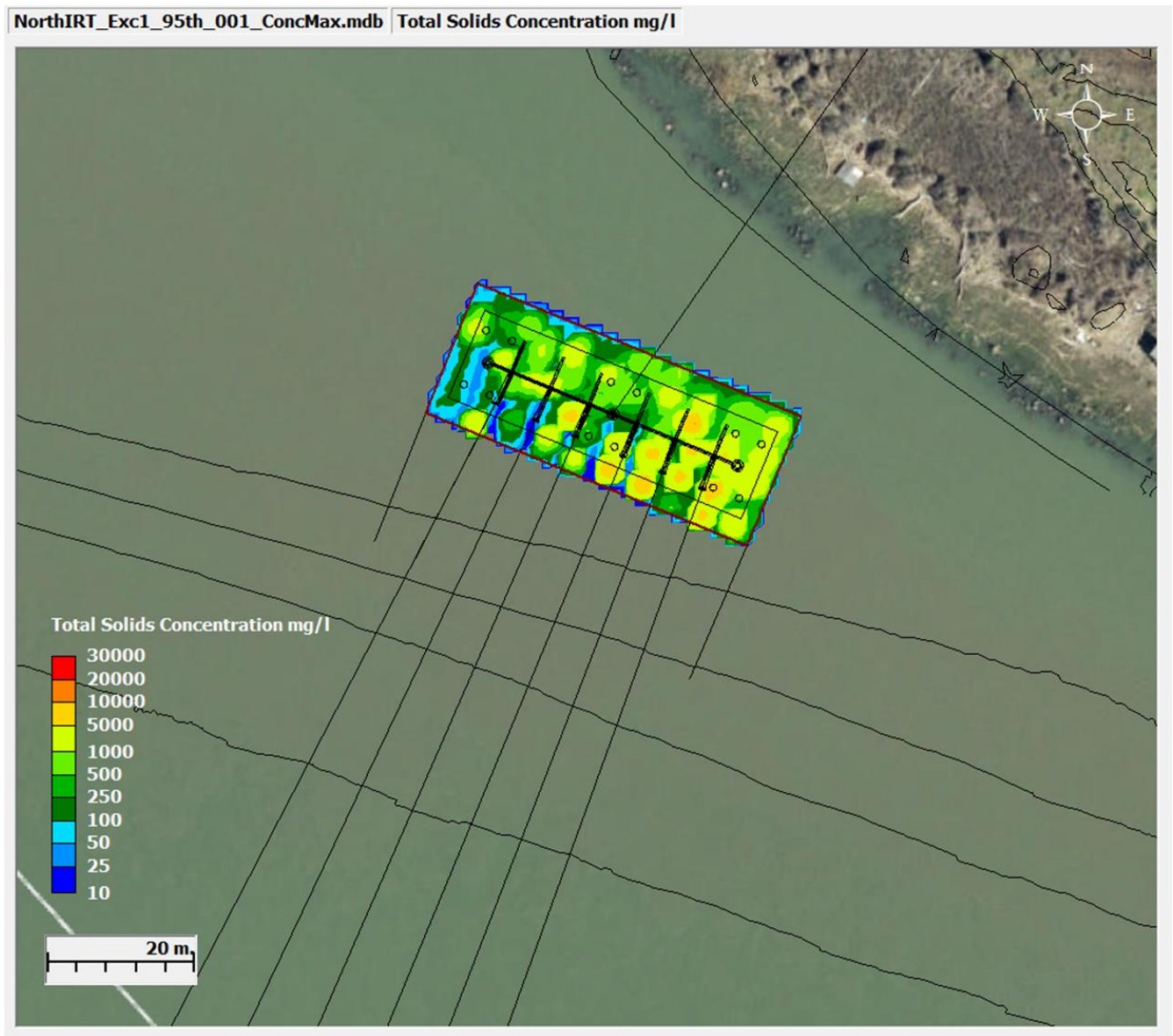
FIGURE 4-5: SCENARIO 4 - MAXIMUM TSS CONCENTRATION DURING R1 EXCAVATION, MAXIMUM CURRENT SPEED
